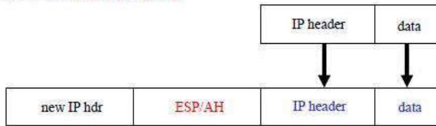
Figure : IPSec Tunnel mode
